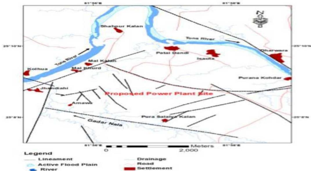
Fig.8: Lineament map of Meja thermal Power Plant Site.
