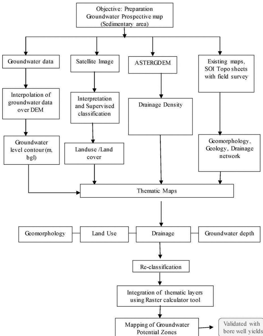
Fig. 3: Schematic flowchart for groundwater potential zone mapping
