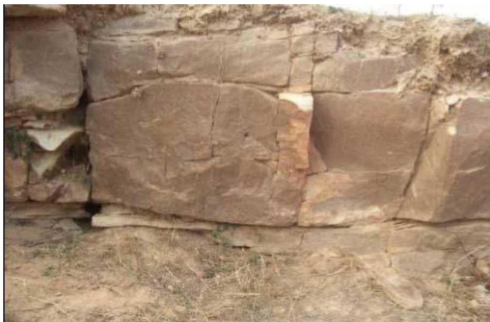
Fig. 2: Blocky nature of rock due to disposition of horizontal and vertical joint sets
